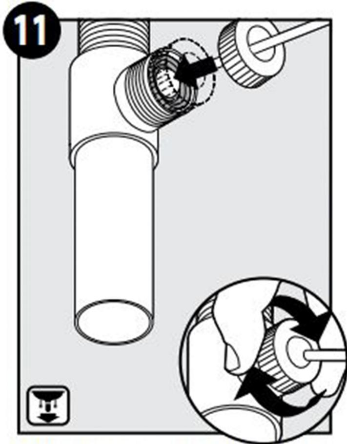
**11** Insert pivot rod into opening and tighten pivot rod nut (P) finger tight.
