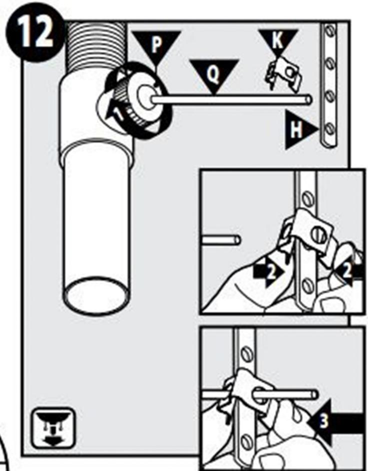
**12** Slide one side of the pivot rod clip (K) onto the pivot rod (Q). Position the pivot rod strap (H) so the pivot rod (Q) passes through one side of the clip (K), through the closet hole on the pivot rod strap (H) and through the hole on the other side of the clip (K). Squeeze the ends of the clip (K) to adjust the positioning and let go to lock.
