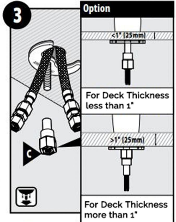
For sinks thinner than 1" attach the mounting nut (C) with the smaller end up as shown. For sinks thicker than 1" attach the mounting nut (C) with the larger end up as shown.
