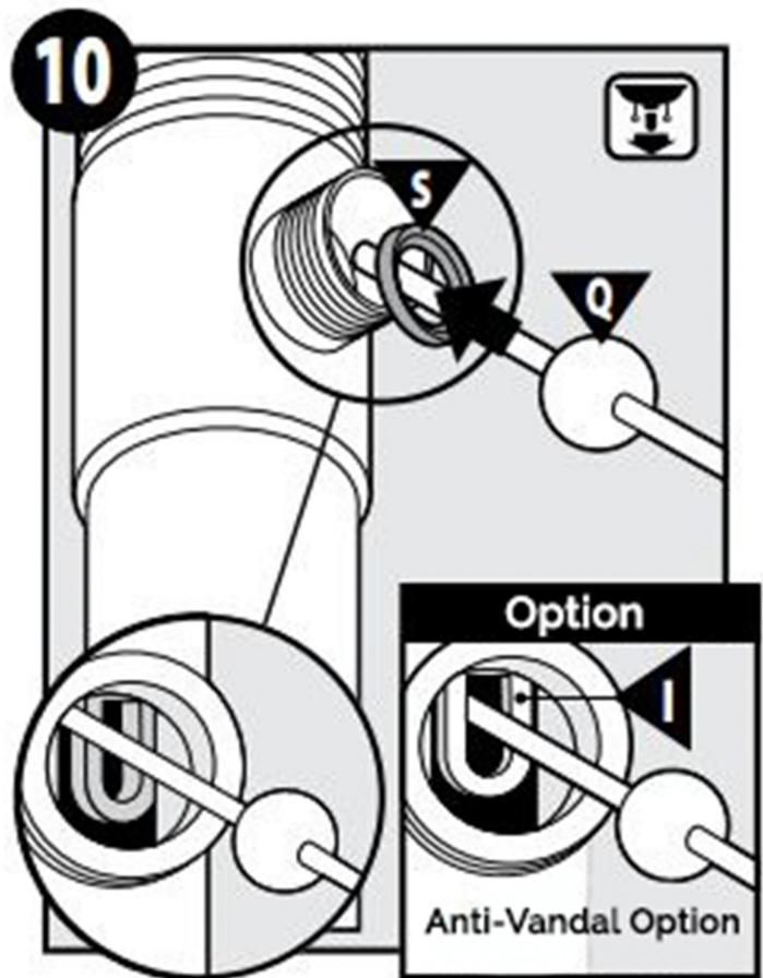
Verify that the white plastic pivot rod seal (S) is in place with beveled side facing out. The pivot rod (Q) can be installed two ways the illustration shows the pivot rod in the EASY CLEAN position which allows the plug to be pulled out for cleaning. The other option (Illustrated in the insert) shows the pivot rod installed in the VANDAL PROOF position. The end of the pivot rod (Q) is inserted into the opening at the bottom of the plug (I).
