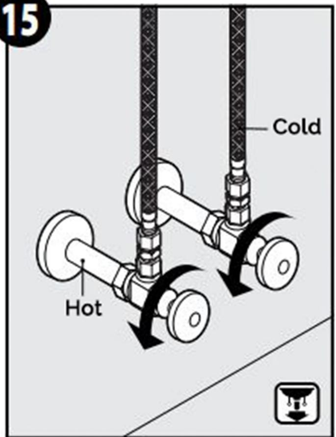
Turn on the water supply line valves on and check for leaks.
