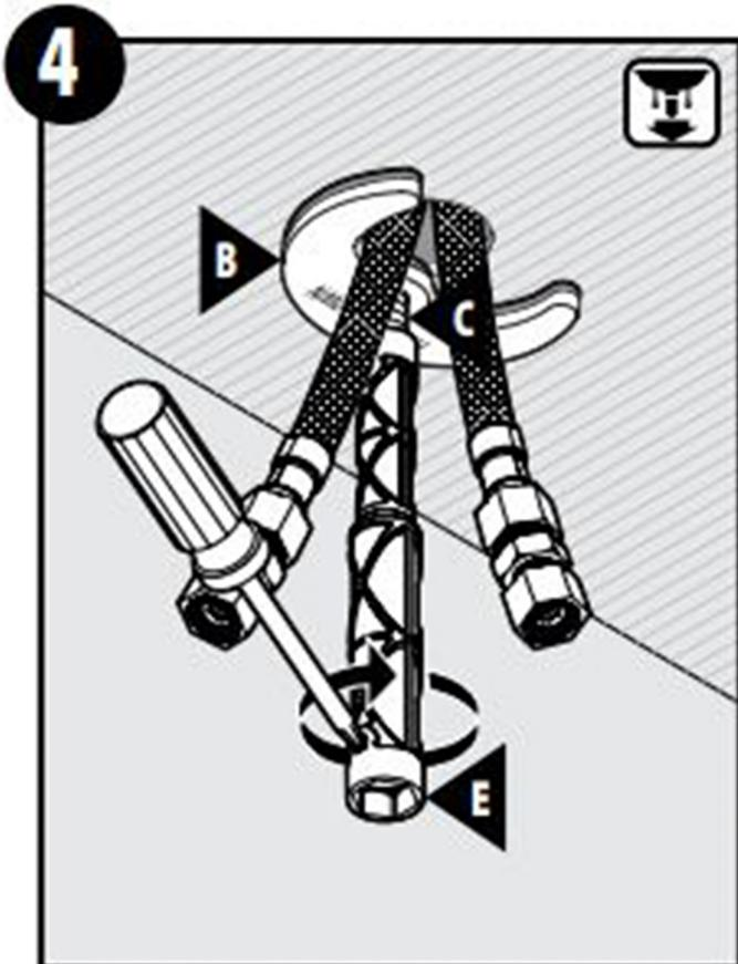
4 Plate the small end of the mounting tool (E) onto the mounting nut (C) and tighten to secure the mounting bracket (B). Insert a screwdriver into the hole and tighten.
